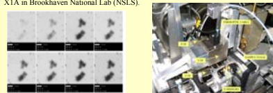
Left: Series of Scanning Transmission X-ray Microscopy (STXM) images of load soot particles, for energies from 282.5 eV to 296.0 eV. Due to X-ray optical contrast, spatial chemical variations allow to assign specific absorption spectra to single particles or even particular sample regions. Right: NEXAFS of single (load soot) particles from Diesel and oxygenated Diesel, as obtained with STXM.
