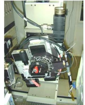
Photograph of the rotational stage for USAXS instrument
