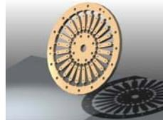
3-D model of the overconstrained weak-link mechanism
